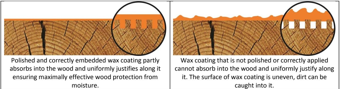
Polished and correctly embedded wax coating partly absorbs into the wood and uniformly justifies along it ensuring maximally effective wood protection from moisture.
